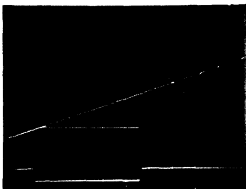
TOP TRACE: INPUT AND SAMPLED OUTPUT SUPERIMPOSED 100\text{ mV/DIV} & 100\text{ ns/DIV} BOTTOM TRACE: SAMPLING SIGNAL 20\text{ V/DIV} & 100\text{ ns/DIV}
